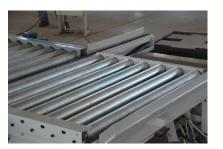
The heavy duty precision side frames are made of heavy gauge sheet metal.
